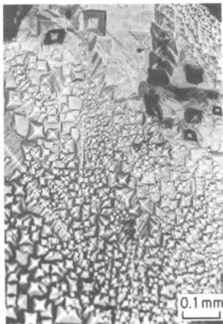
Figure 2 Equidistantly spaced etch pits along grain boundaries in combination with densely populated etch pits.
