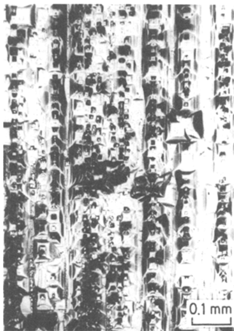
Figure 1 Parallel rows of square etch pits in the [001] direction along slip traces on \{100\} faces.
